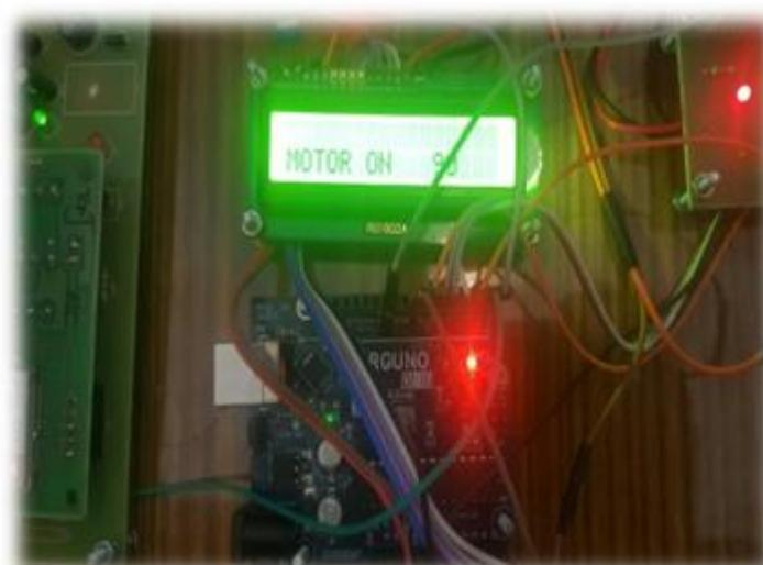
**Figure.4** DC Motor Running and Servo Motor Angle 90°
