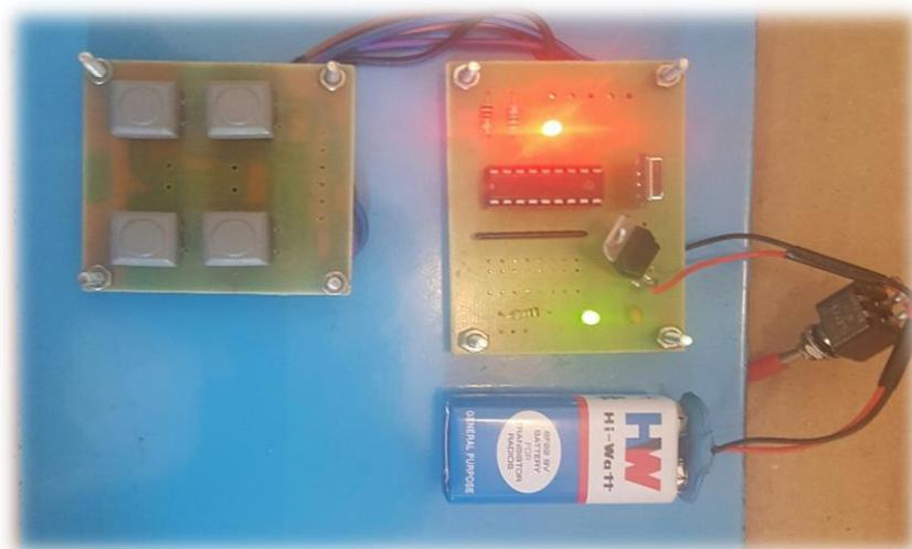
**Figure.3** Remote Control Unit of the Prototype
